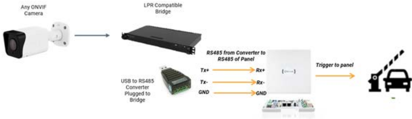
Figure 111. Connection between the Eagle Eye Bridge to the Brivo Panel using an USB to RS485 converter
