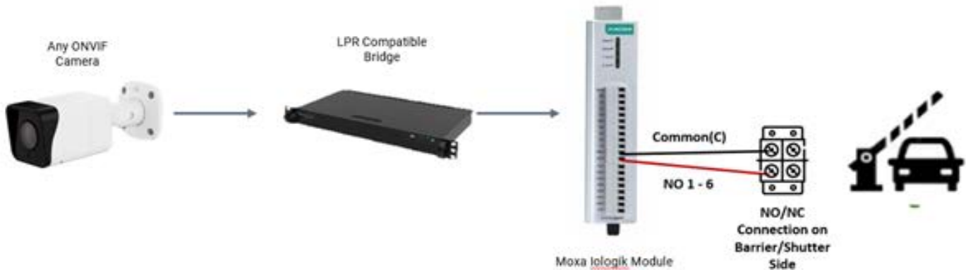
Figure 115. Moxa Connection to a Barrier/Shutter
